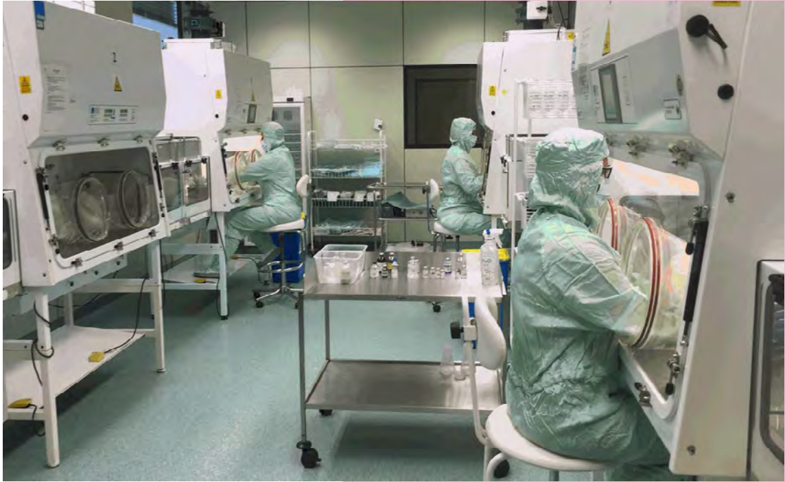
Figure 10-2: HMP preparation in isolators (externally vented) at the Masaryk Memorial Cancer Institute, Czech Republic
