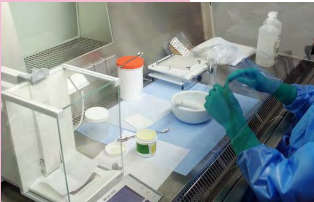
Figure 10-6: Capsule production in a BSC at Pharma Assist BV, The Netherlands. Using HMP powders is a high-risk activity that has the potential to generate airborne particles.
