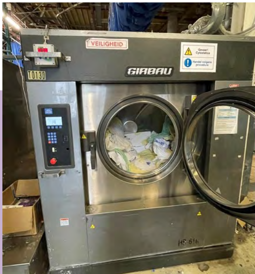
Figure 14-4: A separate first wash of HMP-contaminated laundry. Single-use laundry bags are washed together with the laundry prior to disposal. Source: Rentex, The Netherlands
